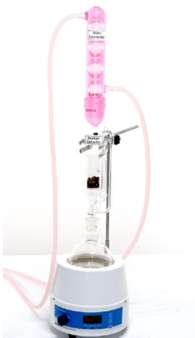
3. Soxhlet Extractor Setup (complete)
