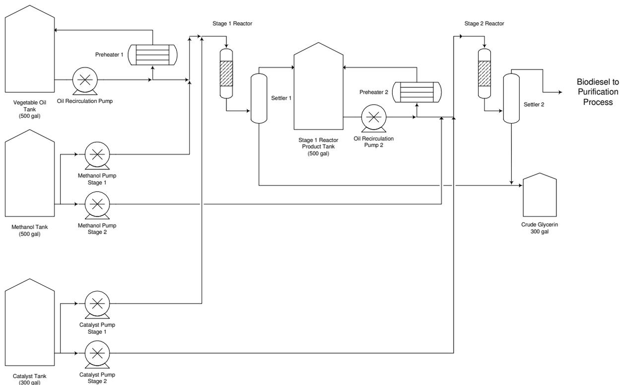
Figure 1 - Process Flow Diagram – 2-stage biodiesel process
